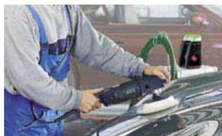
All switches within easy reach. The speed range of 0 to 2400 rpm (via accelerator switch) widens the application range considerably.
